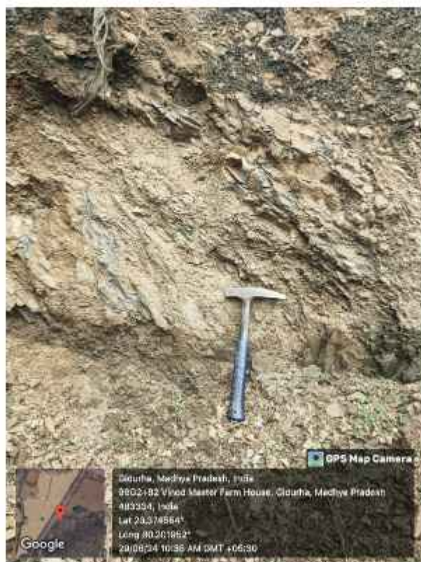
Photo 3.1. Soft Laminated ore, Specularite present near Gidurha village. Sample location-MJP-01
